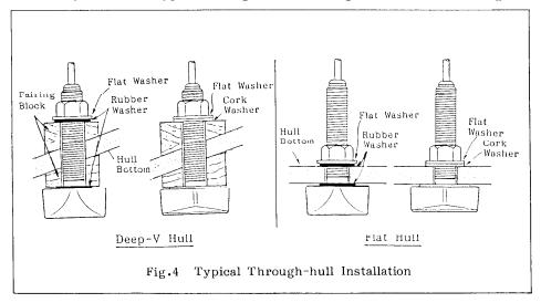
Through-hull mounting is accomplished as follows.
